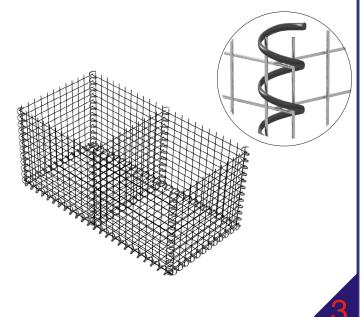
18" Stiffeners or lacing wire should be placed inside at 12" intervals (, per WV) WMUFX) and secured over the line UbX cross wires on the front and side ZUWY "None are needed in interior cells.
